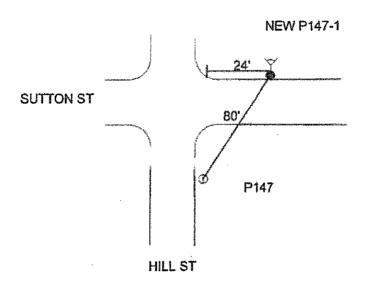
NGRID TO INSTALL A 40'3 POLE FOR AN OVERHEAD TO UNDERGROUND CONNECTION TO CUSTOMER'S UNDERGROUND SECONDARY FOR A TRAFFIC LIGHT
