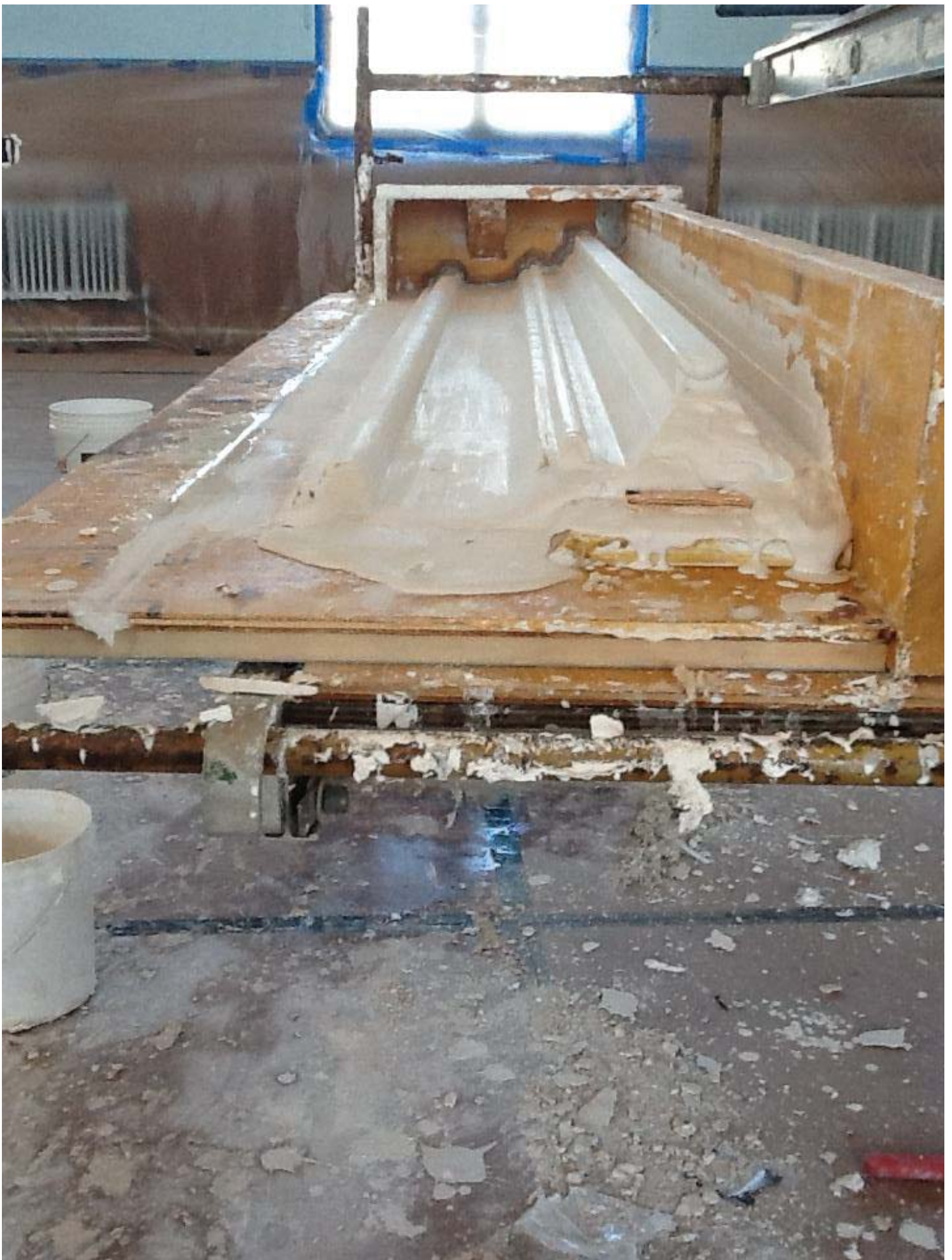
3. Close-up showing wet plaster of a recently drawn section of molding
